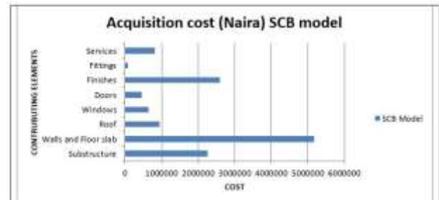
Figure 1: Capital cost of the SCB building model
