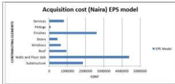
Figure 2: Capital cost of the EPS building model
